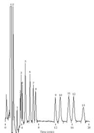
Fig 2.7 Chromatogram obtained with Electrochemical Detector
